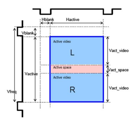
Note that the active area between the left and right eye data is not required and should not be used unless required by the video source.
